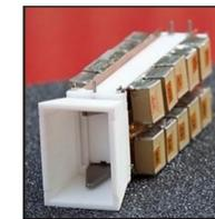
Above: Mars Space Ltd.'s Micro-PPT for NanoSats<sup>5</sup> that produces 562 m/s of  $\Delta V$ . Right: Busek's BmP-220 PPT<sup>6</sup> that produces 438 m/s of  $\Delta V$ .
