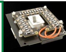
Above: Clyde Space's CubeSat  $\mu$ PPT<sup>3</sup> that produces 296 m/s of  $\Delta V$ . Right: Clyde Space's CubeSat PPT<sup>4</sup> that produces 151 m/s of  $\Delta V$ .
